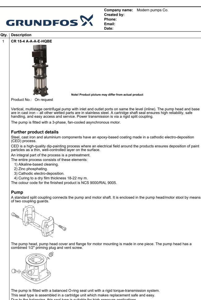
Due to the balancing, this seal type is suitable for high-pressure applications.
